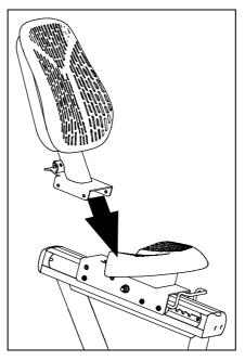
Figure 7: Positioning the seat back assembly
